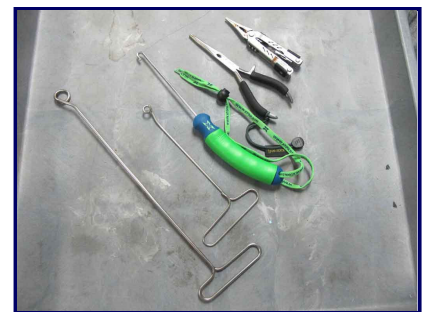
(De-Hooking.JPG) L-R two ARC dehookers, the X-Tool J-dehooker, and long-nosed fishing pliers. Click to enlarge.
